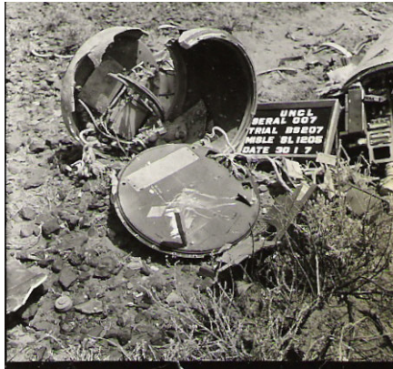
Figure 5: an experiment after landing - another parachute failure
